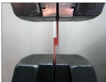
Fig 4: testing the samples by using the universal testing machine
