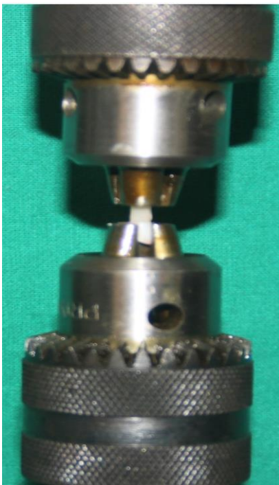
Fig 11: Specimen under microtensile bond strength testing
